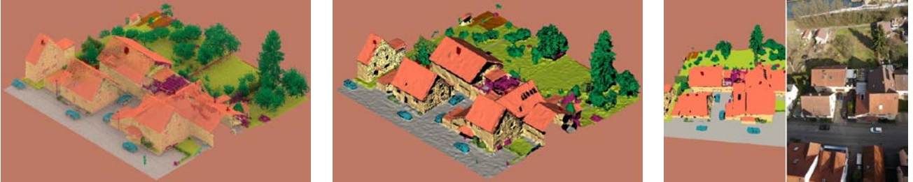
Fig. 1: The explicit linking of pixels, points, and faces (multi-modal data fusion, see Table 1) enables the consistent information exchange across the three modalities point cloud ( left ), mesh ( center ), and imagery ( right ). The figure exemplarily depicts the automated label propagation from the manually annotated point cloud to the mesh and an oblique image (for a subset of Hessigheim 3D (KÖLLE ET AL. 2021)). Faces that cannot be linked to points remain without a label (depicted in black ). Pixels that are linked to an unlabeled face are colored in black . Background and non-associated pixels are colored in reddish-brown .
